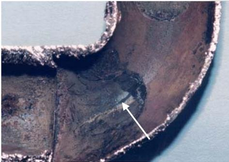
**Fig 3** – Close-up view of crack (see arrow) which initiated in residual flux puddle.
