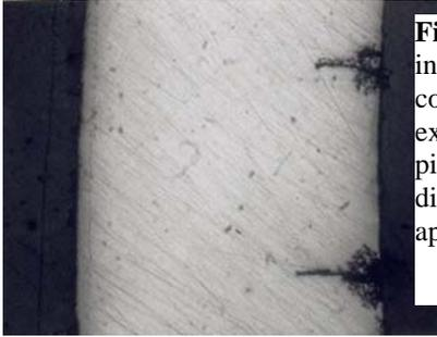
**Fig 2** – Copper pipe wall in section. Typical corrosion fatigue cracks extending from corrosion pits on the internal diameter. Magnification approximately 65 X.
